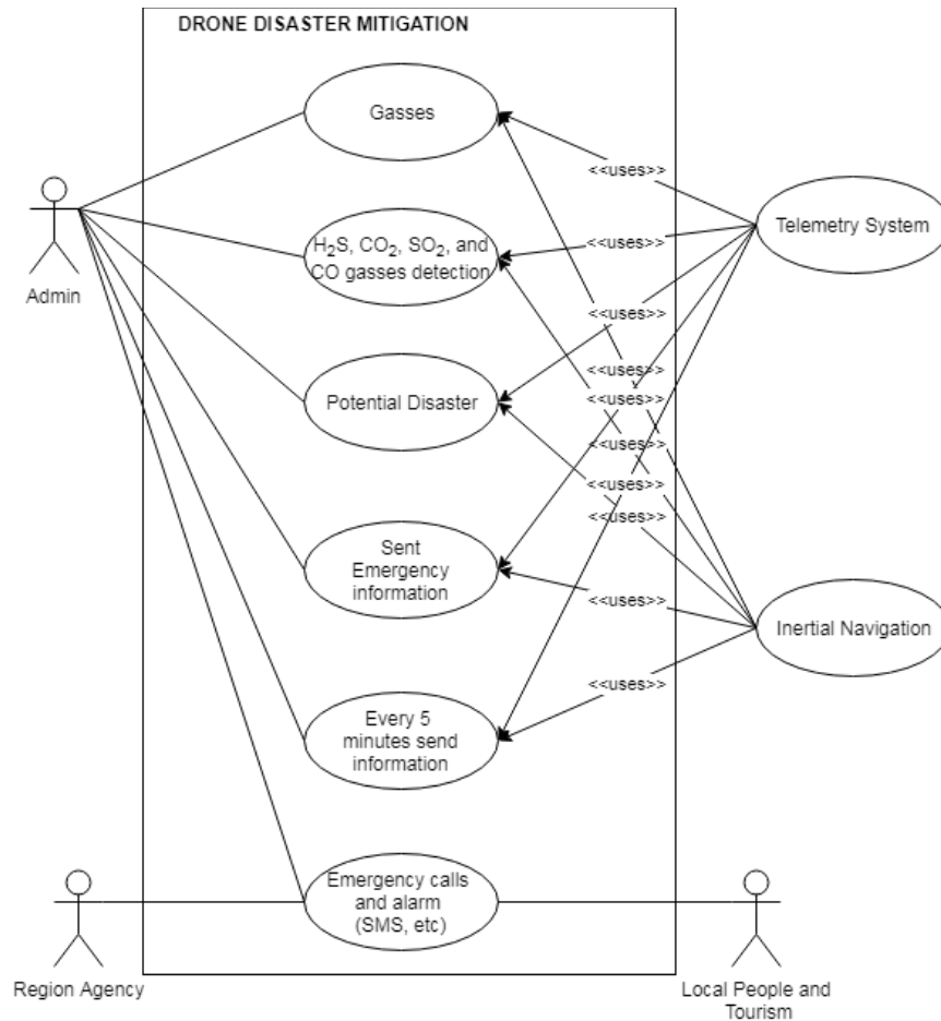
Figure 2. UML Implementation of operational mechanism EWS mitigation ecotourism via Drone.
