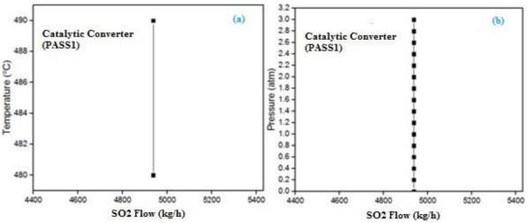
Figure 3: SO<sub>2</sub> Mass Flow Response to Temperature and Pressure Variation
