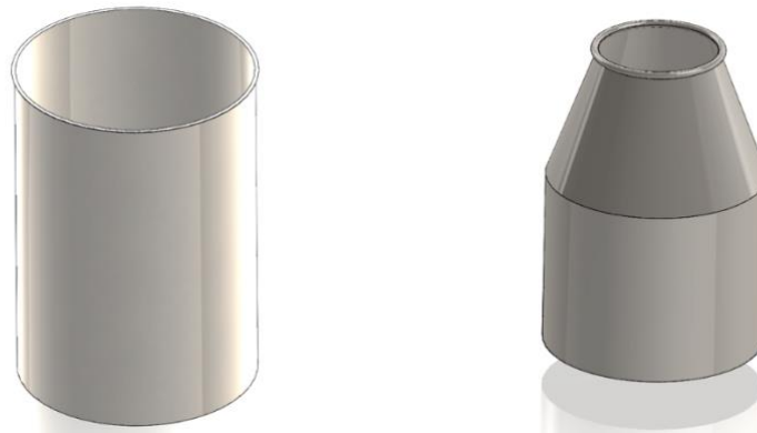
Figure 3. Milk can design model (a) regular tube and (b) cone dome tube
