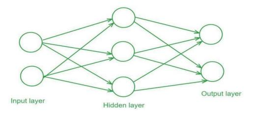
Figure 2. Feedforward neural network architecture
